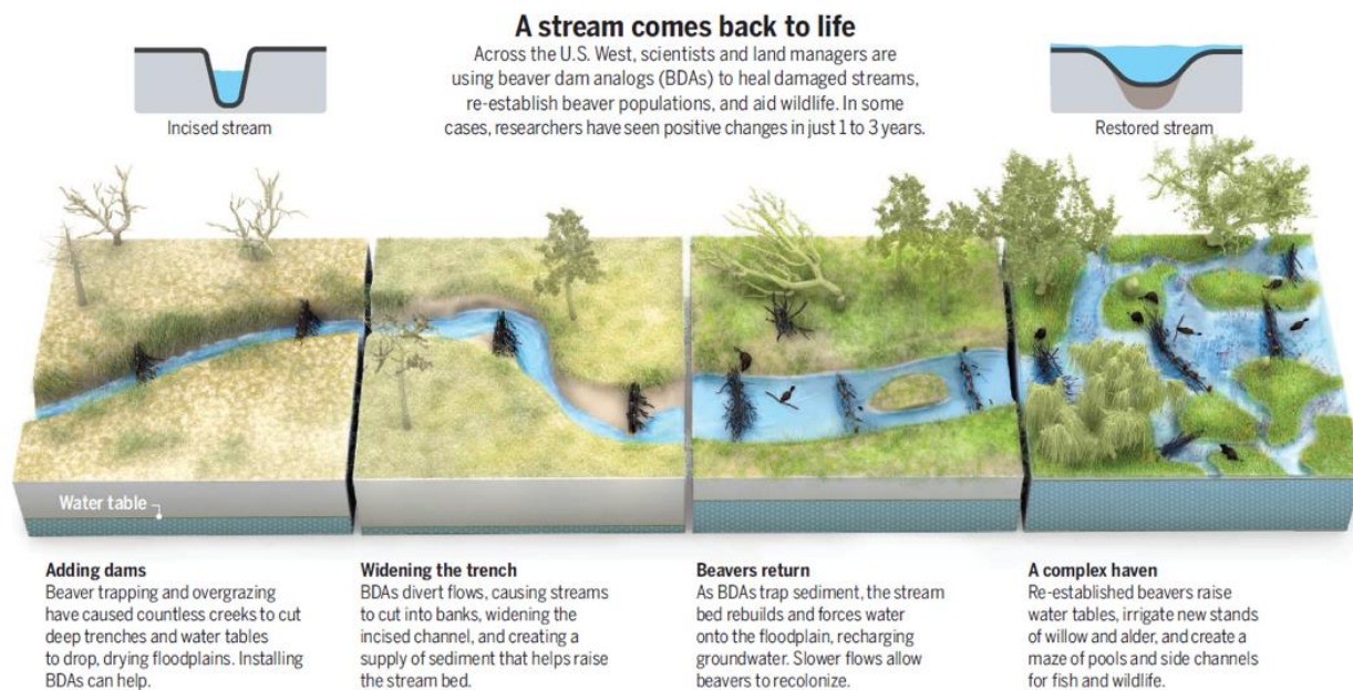
Figure 4. Illustration of the process of encouraging beaver dam activity with beaver dam analogs (i.e., a man-made structure designed to mimic the form and function of a natural beaver dam) and how this can lead to (on right) self-sustaining conditions. Source: Goldfarb, 2018. 13
