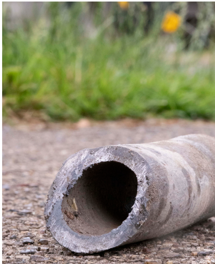
Part of a lead service line removed from outside a home in Chicago, Illinois.
