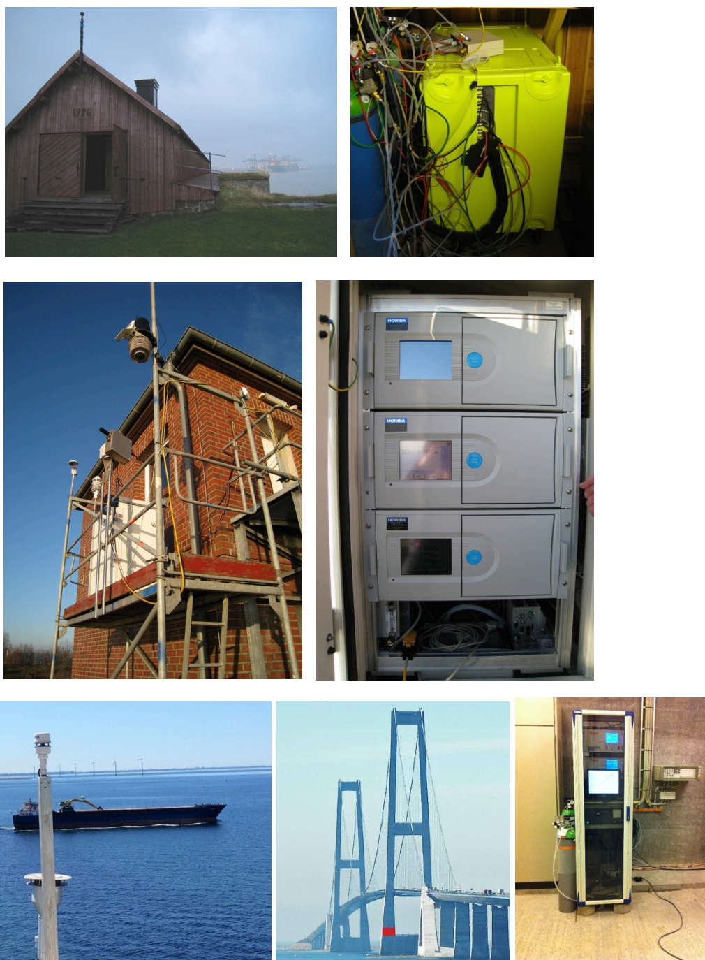
Figure 6. Fixed-point sniffer devices near the Port of Gothenburg in Sweden, the Port of Hamburg in Germany, and on the Great Belt Bridge in Denmark
