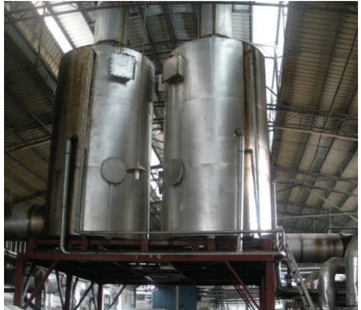
Heat recovery from setting machine exhaust gas
