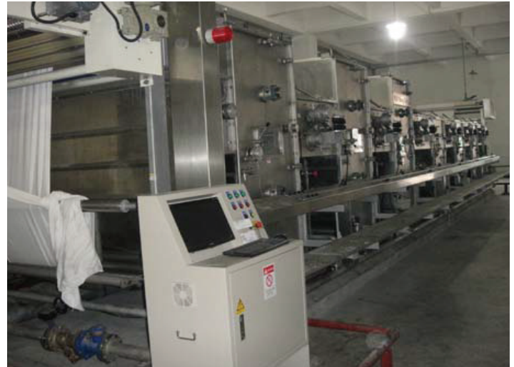
The new type of continuous oil removing and scouring/rinsing machine
